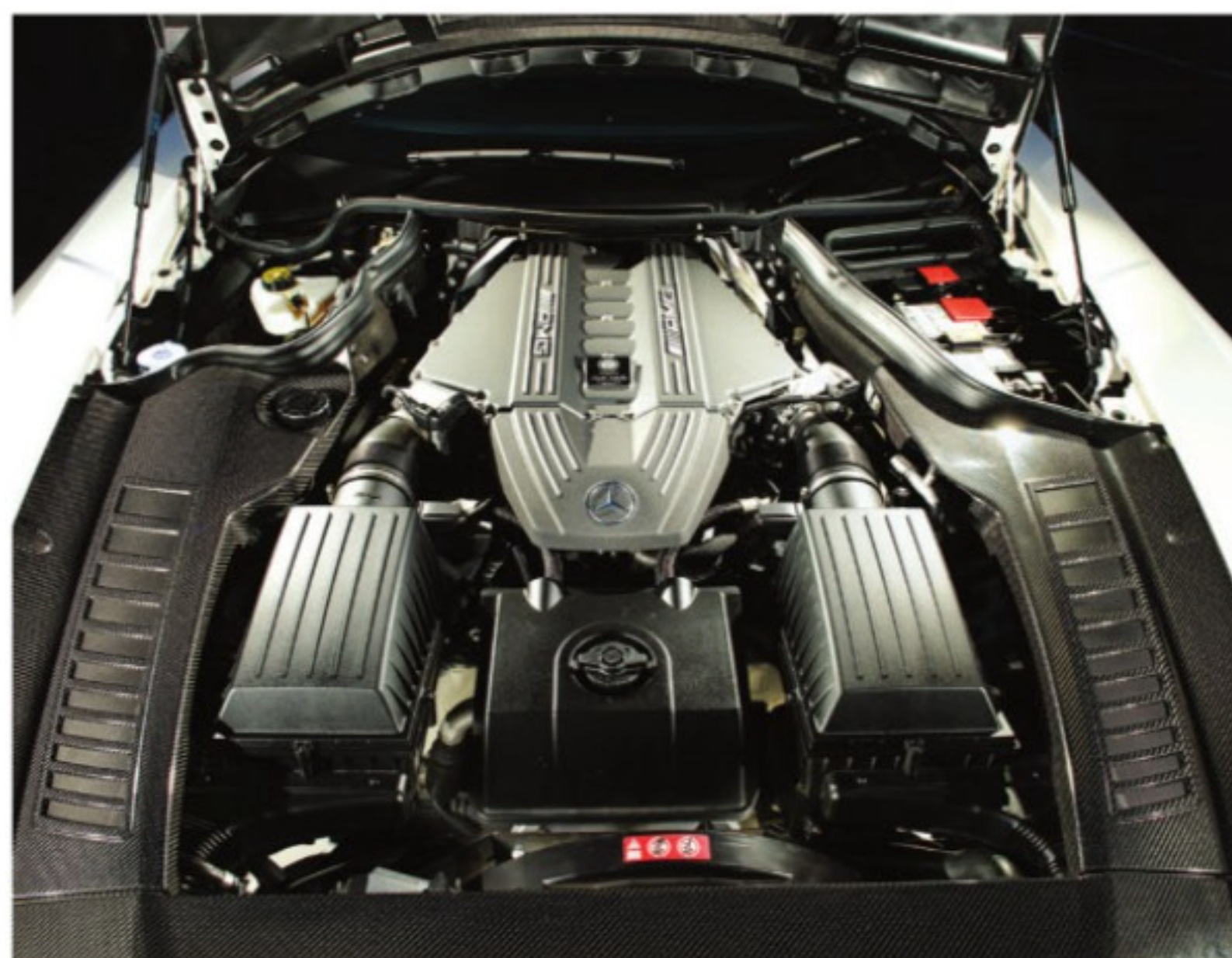
◁ The M159 V8 with four cams, two headers and dry sump lubrication.
